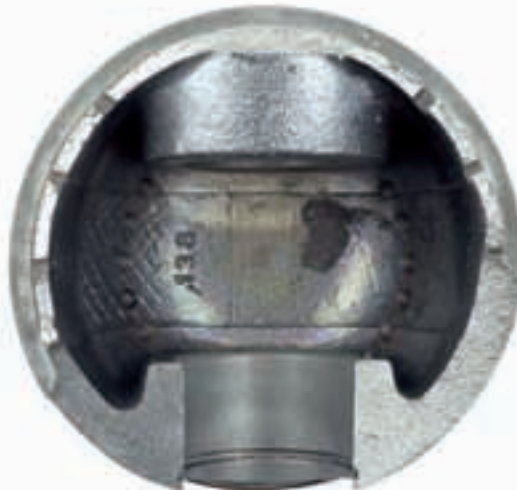
Fig. 3 Piston snapped off at a right angle at the height of the piston pin axis
