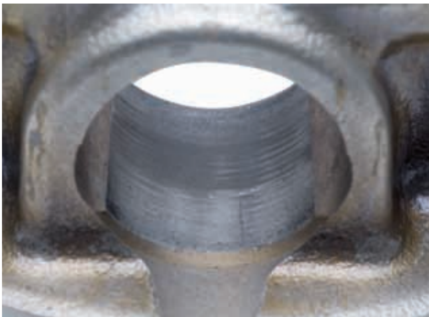
Fig. 3 Pin bore with seizure marks
