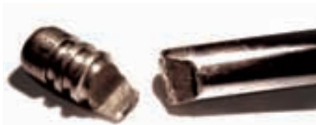
Fig. 2 Valve base broken in the groove (overload fracture/bending stress)
