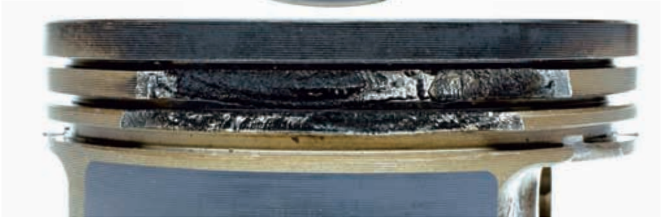
Fig. 2b Close-up view of the broken piston ring lands
