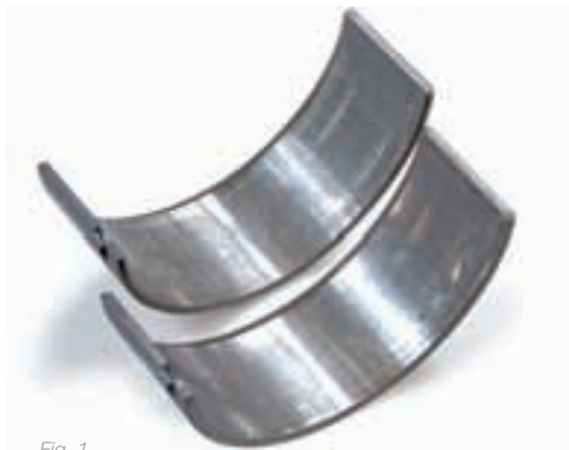
Fig. 1 Shiny marks on the running surfaces of the bearings
