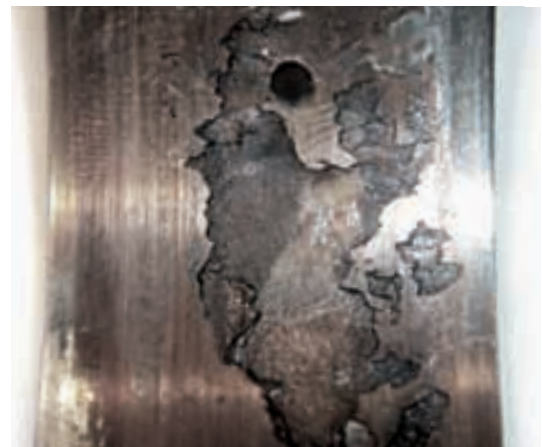
Fig. 1b Close-up view of the damaged bearing layer
