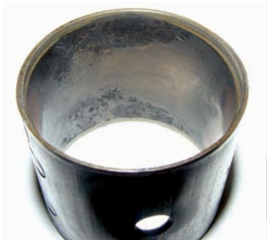
Fig. 2 Damaged connecting rod bushing
