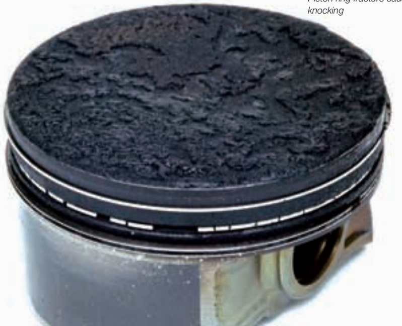
Fig. 4a Piston ring fracture caused by knocking
