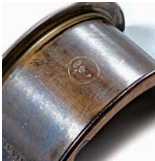
Fig. 2 Contamination imprint on the outer surface of the bearing
