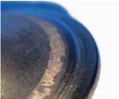
Fig. 1 Heavy wear on the sealing surface
