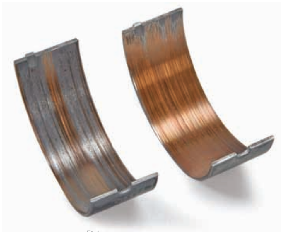
Fig. 1 Heavy scoring in circumferential direction
