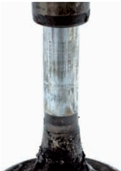
Fig. 1b Clearly visible in the close-up view: Deposit build-up and seizure marks on the valve stem
