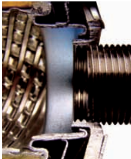
Fig. 2 Incorrect thread length due to loose conternut
