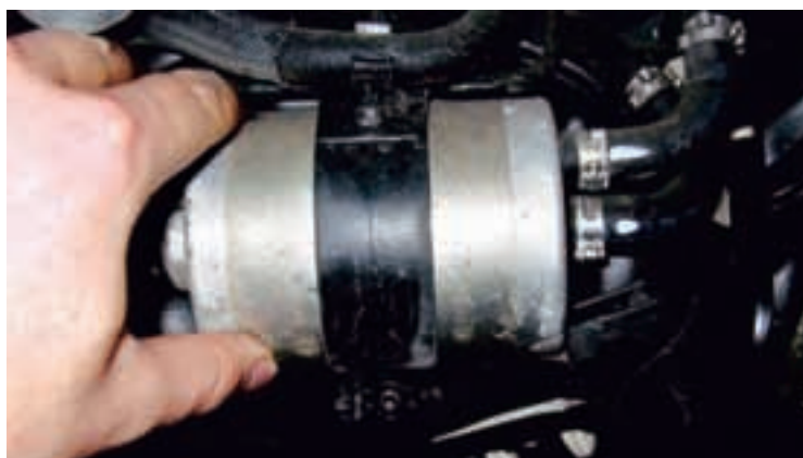
Fig. 6 Contact corrosion due to damaged insulation
