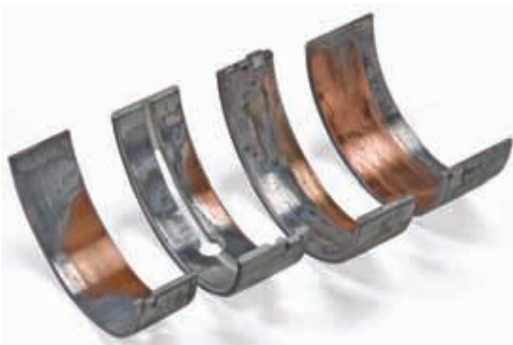
Fig. 1 Uneven wear at the bearings
