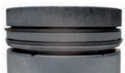
Fig. 2 Heavy axial wear particularly at the top ring
