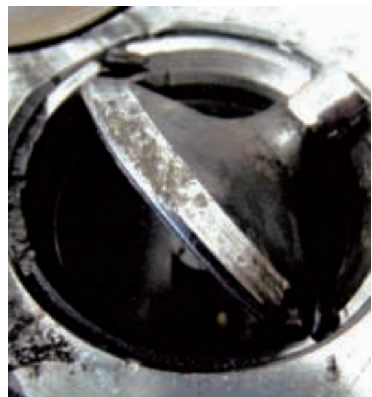
Fig. 1 Snapped off valve in the valve head area
