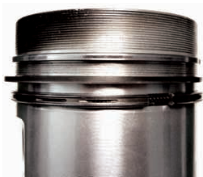
Fig. 2 Top land with irregular deposits
