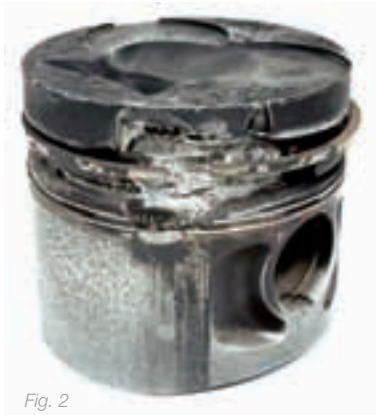
Fig. 2 Ring belt with shiny surface
