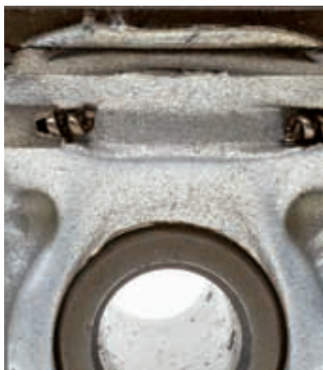
Fig. 1b Close-up surface view of softer piston material and harder piston ring material worn to the same extent
