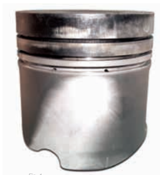
Fig. 1 Asymmetrical wear pattern (slanted position) at the piston skirt
