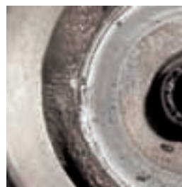
Fig. 5 Marks at the cylinder head caused by an incorrectly inserted valve spring
