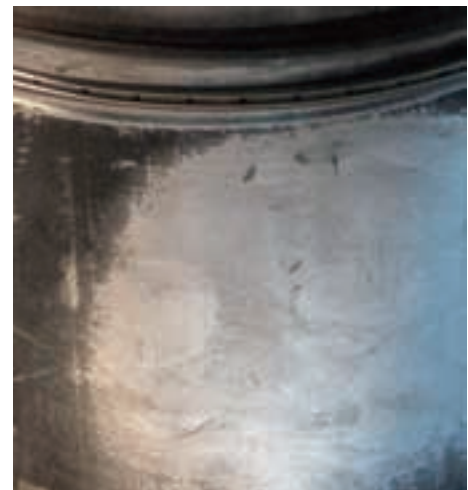
Fig. 1 Wide wear pattern and scoring marks due to fuel dilution
