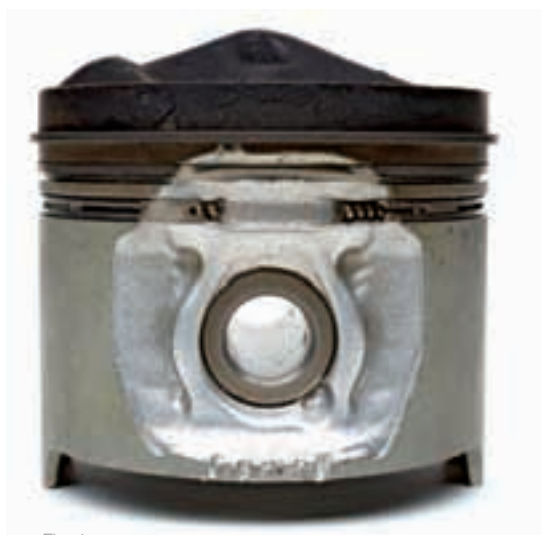
Fig. 1a Cratered piston wall, caused by a loose piston pin circlip or contamination in the piston pin
