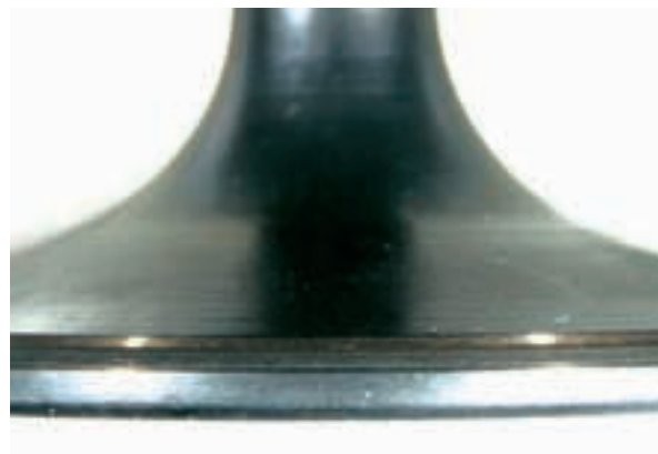
Fig. 2 For comparison: Valve head without deformation
