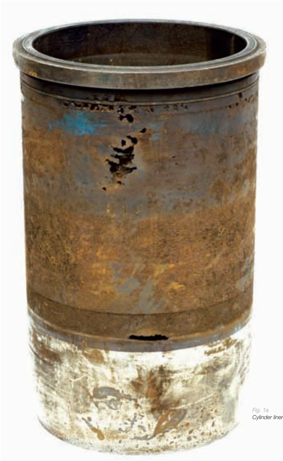
Fig. 1b Close-up view of the cylinder liner with sharp edges and cavities which become larger towards the inside
