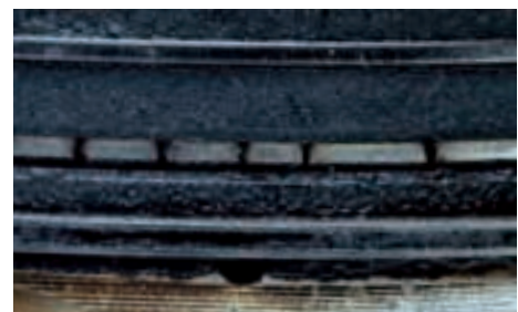
Fig. 4b Close-up view of a piston ring fracture
