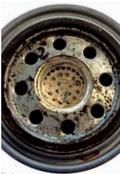
Fig. 1 Granules escaping from the air dryer cartridge
