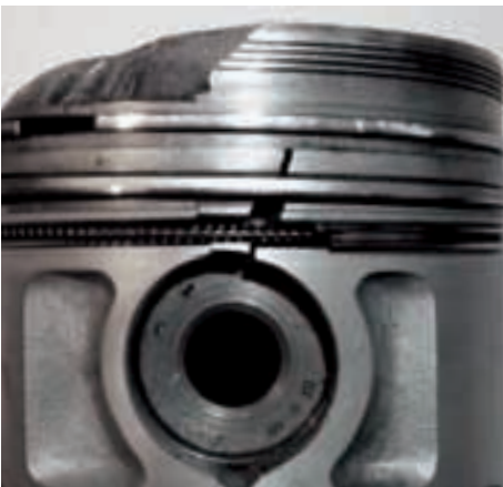
Fig. 3a Overload fracture from the top of the piston to the pin bore
