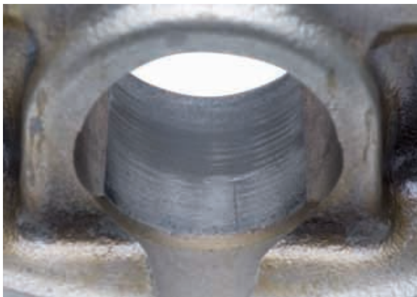
Fig. 1 Seizure in the pin bore
