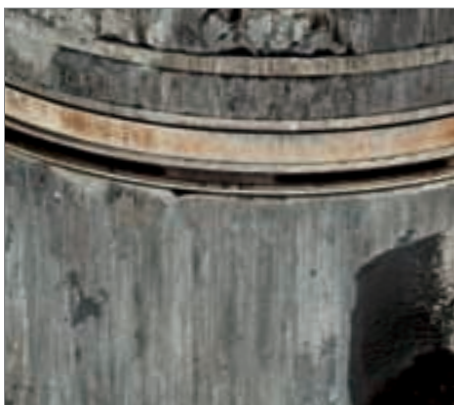
Fig. 2 Piston rings with burn marks
