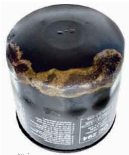
Fig. 4 Damaged coating – the result: Corrosion
