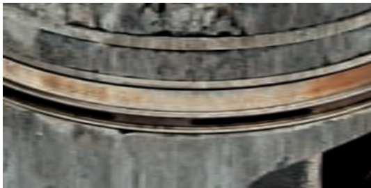
Fig. 2 Scoring marks and burn marks on the piston rings
