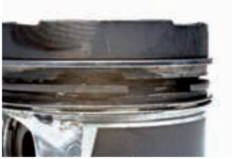
Fig. 1 Heavily worn piston ring groove
