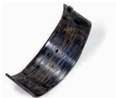
Fig. 2 Heavily worn and spun bearing
