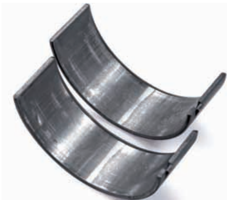
Fig. 1 Worn outer edges of a bearing
