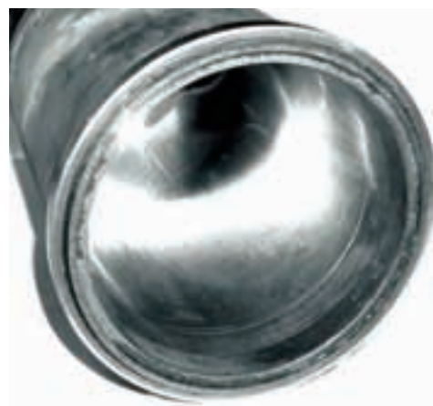
Fig. 3 Worn cylinder liner
