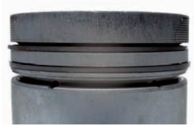
Fig. 4 Axial wear at the piston rings
