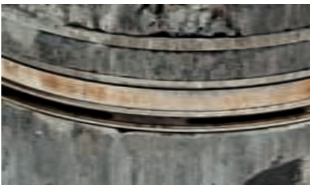
Fig. 2 Scoring marks and burn marks on the piston rings
