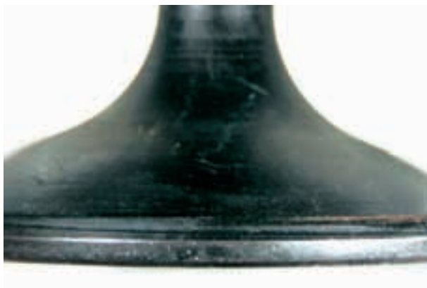
Fig. 1 Deformed valve head (tulip-shaped)
