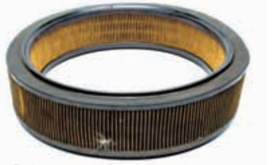
Fig. 3a Extremely dirty air filter element, filter change imperative
