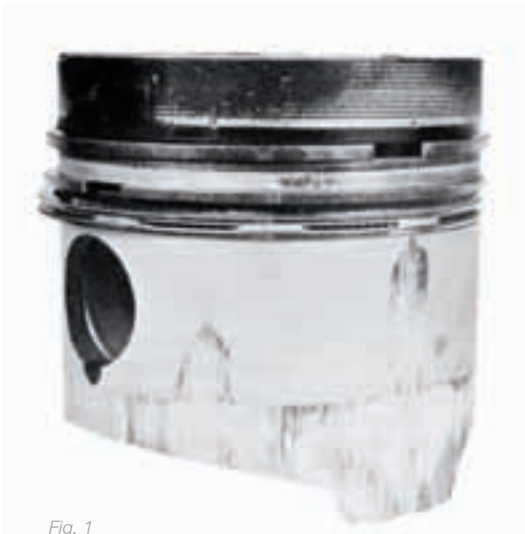
Fig. 1 Seizure at the lower piston skirt due to constriction of the cylinder liner
