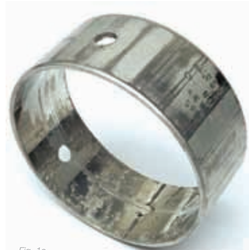
Fig. 1a Pitting caused by mechanical overload or inadequate load-bearing ability of the oil film
