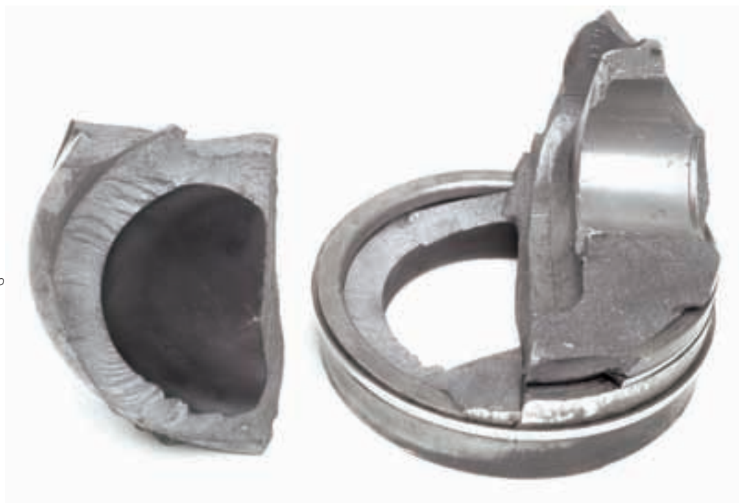
Fig. 1 Broken commercial vehicle piston due to hydraulic lock
