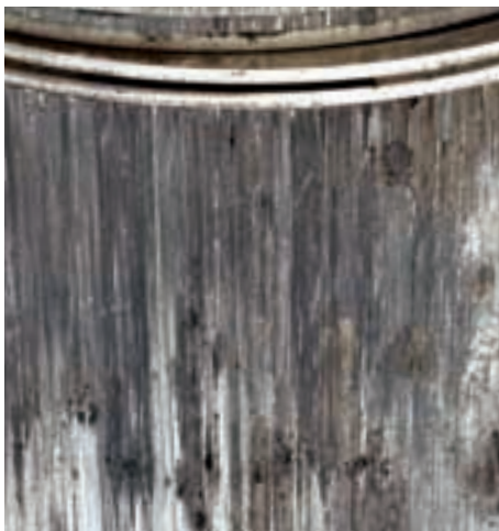
Fig. 1 Seizure only on the thrust side of the piston skirt
