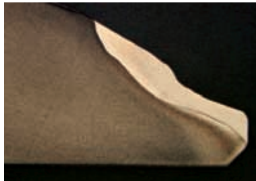
Fig. 3 Heavily worn sealing surface (stellite hardened)
