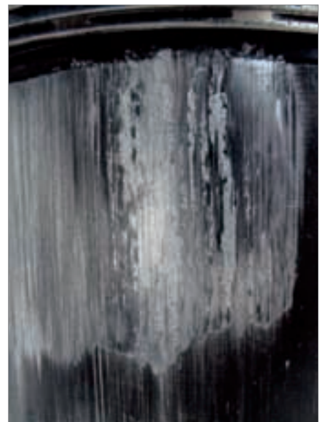
Fig. 2 Partially shiny seizure marks
