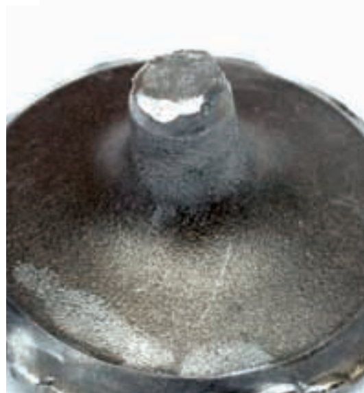
Fig. 3 Vibration fracture with fracture surface at the valve stem
