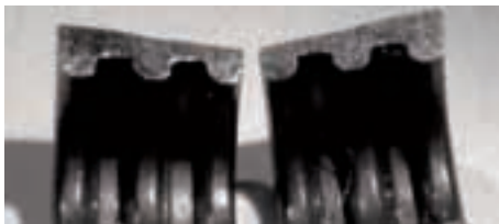
Fig. 3 Deformation of the valve keepers at the ribs
