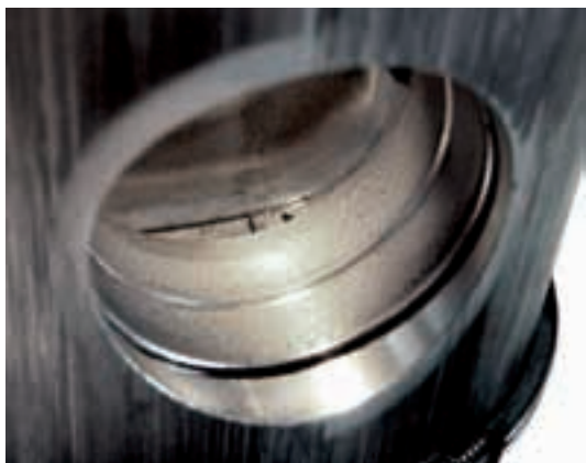
Fig. 4a Pitting in the pin bore due to diluted engine oil
