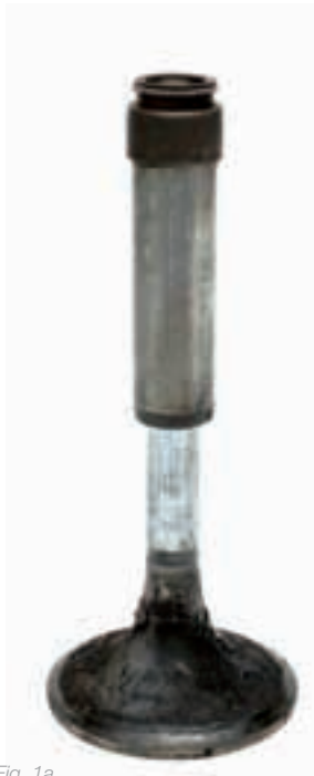
Fig. 1a Valve with seizure in the guide
