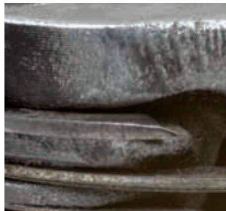
Fig. 1 Erosion at a gasoline piston
