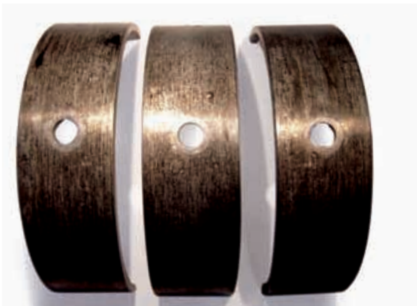
Fig. 1 Shiny marks on the outer surface of the bearing
