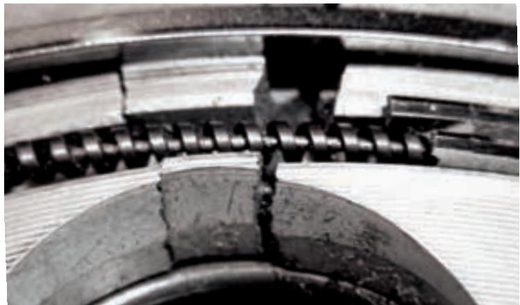
Fig. 3b Close-up view of an overload fracture
