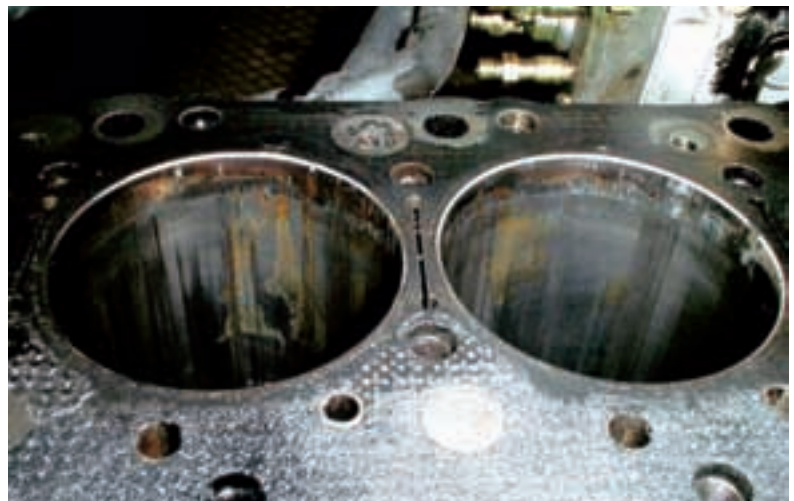
Fig. 2 Cylinder bore with longitudinal scoring marks
